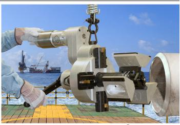
The clamping system of the Commander MILLHOG® Model C-314 pipe beveling machine has six contact points that minimize vibration for chatter free bevels on both thin and heavy wall pipe.
