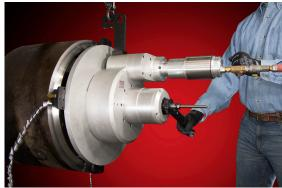
Compound bevel, face, and bore on 24" carbon steal pipe, 2" wall and wall variance of 1/4"
