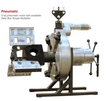
The patented Dual Spring Hanger and Safety Chain provide a perceptible feel that the tool is aligned to the pipe as the clamps tighten. The safety chain prevents the possibility of over extending the spring and provides a failsafe catch should the springs fail.
