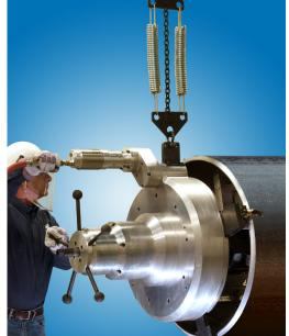
The Terminator MILLHOG<sup>®</sup> Bevels all pipe alloys at any angle for precision fit-up on wall thicknesses up to 2.5" (63.5 mm) using formed tool bits.
