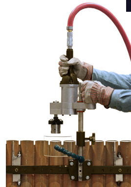
The Standard APS can also achieve perfect cuts on contoured and cylindrical structures, steel plate and pipe from 6.0" to 60.0" with available accessories.
