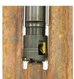
Remove membrane from between tubes
