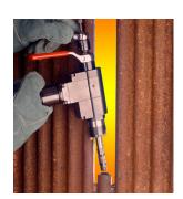
Only 1.5" wide for single boiler tube beveling
