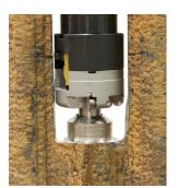
Remove membrane and overlay/ cladding from between tubes
