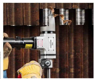
The FIN MILLHOG<sup>®</sup> rack and pinion feed has a 4.0" of stroke that allows the operator to quickly engage and disengage the cutter for clearing separated fin from the work area.
